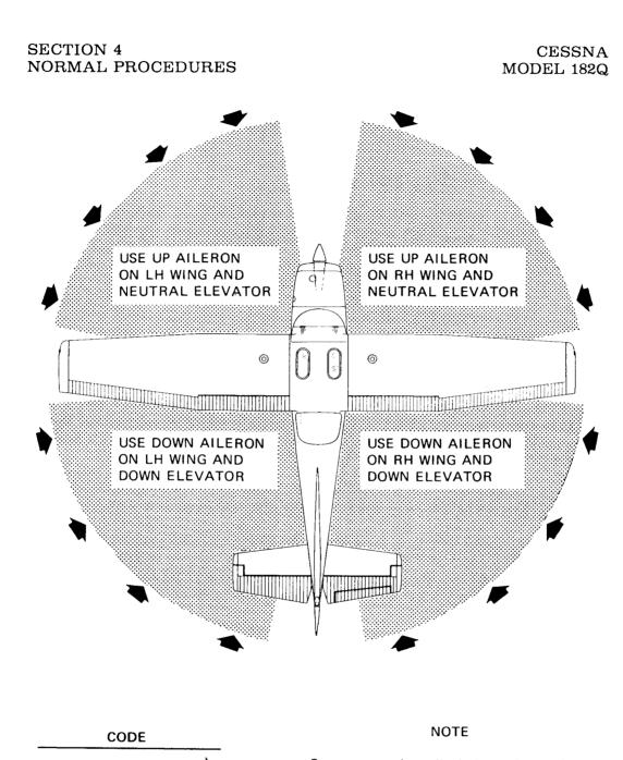
Strong quartering tail winds require caution. Avoid sudden bursts of the throttle and sharp braking when the airplane is in this attitude. Use the steerable nose wheel and rudder to maintain direction.
