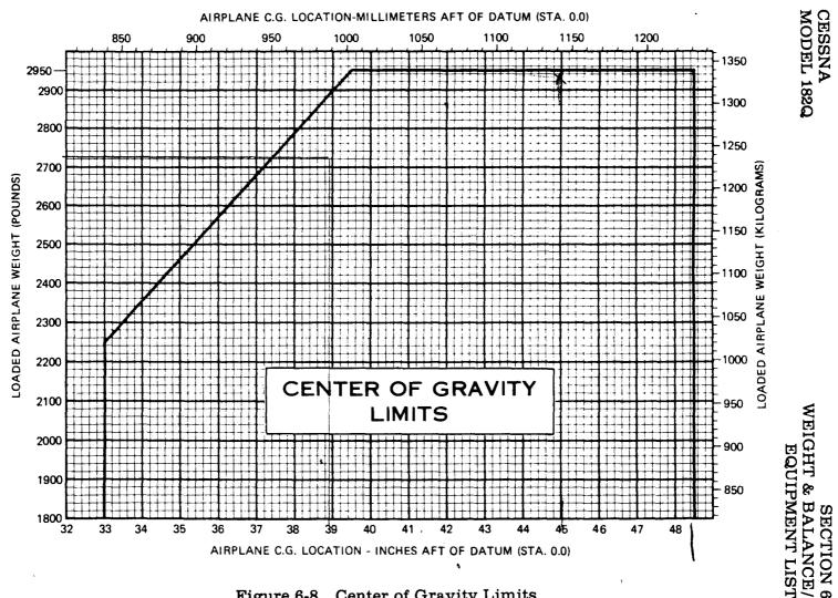
Figure 6-8. Center of Gravity Limits
