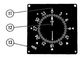
Figure 1. Cessna 400 ADF Operating Controls and Indicator (Sheet 1 of 2)
